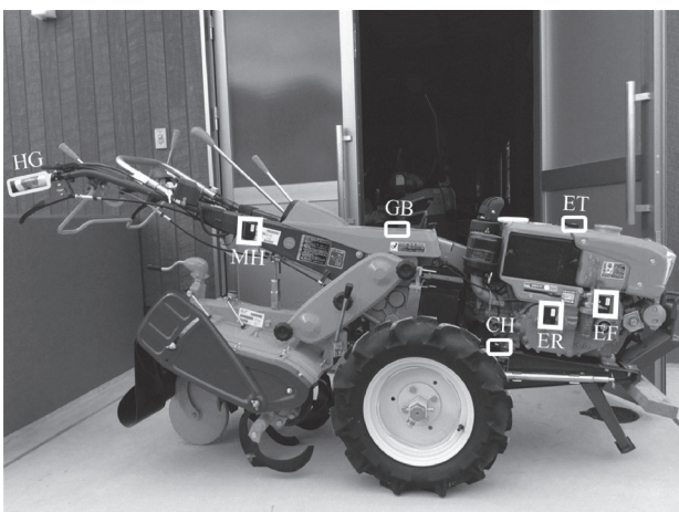
Fig. 1 Experimental hand tractor and sensor allocations
